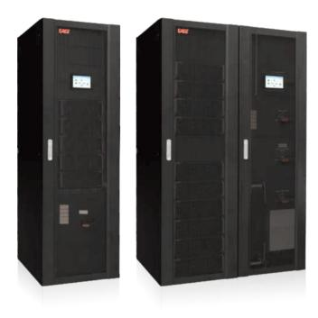
EA660 is the third generation of three phase high frequency on-line double-conversion modular UPS. Its single unit is extendable to 800 KVA, system capacity can be expanded to 3.2 MVA constructed by each power module 50 KVA. All internal modules (Power module, bypass module and control module) are modularly designed and hot-swappable.
