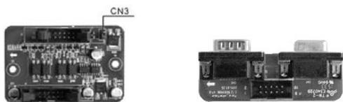
Short circuit cap of parallel card Parallel port board
